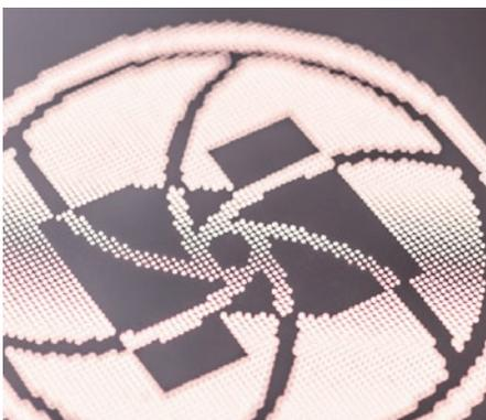
Micro-perforation ( $\phi 0.02$ -mm holes  $\times$  4,000)
